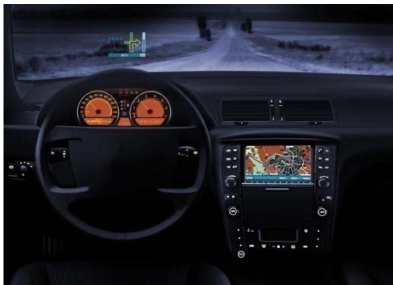
FIGURE 14: UN GPS, ICI AVEC UN AFFICHAGE TETE HAUTE (PROJECTION SUR LE PARE-BRISE). BIEN QUE CONÇU POUR ETRE UNE AIDE A LA CONDUITE, CE TYPE DE DISPOSITIF NECESSITE UN TEMPS D'APPRENTISSAGE POUR L'UTILISATEUR.
