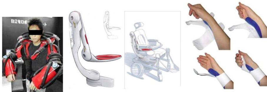
**Fig. 4.** An existing powered orthosis (left), our design (center, here mounted on a wheelchair) and the “glove” control interface (right).
