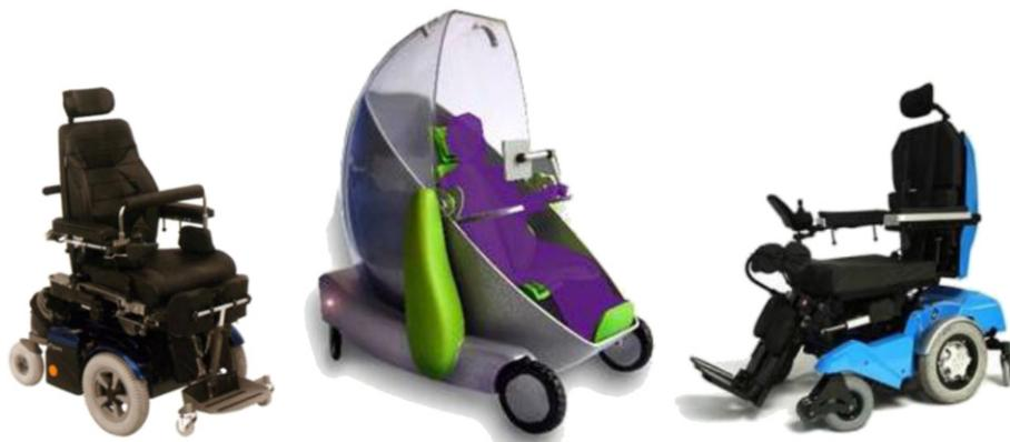
**Fig. 5.** An existing electrical wheelchair (left), one of our concepts (center) and the final WHING (right, here a blue model). (For interpretation of the references to colour in this figure legend, the reader is referred to the web version of this article.)
