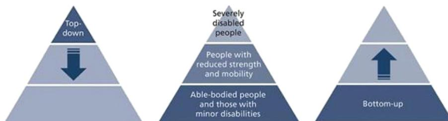
Fig. 2. Top-down and bottom-up approaches in Universal design.
