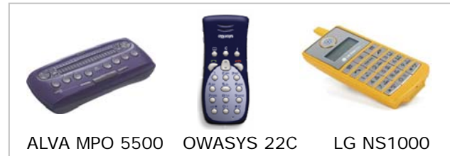
figure 2. Device with Braille interface (left), screenless phone with text-to-speech (middle) and large keypad (right).
