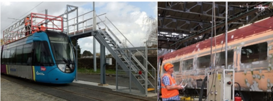
Fig. 1. Inspection of a box roof via a walkway (left) vs. with a drone (right).
