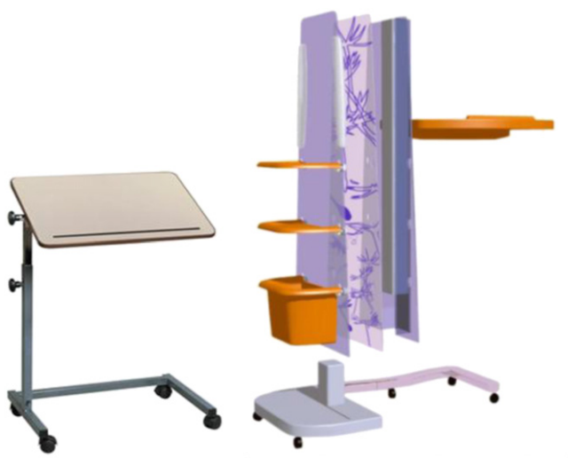
Fig. 3. An existing overbed table (left) and our design (right, exploded view).
